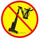
Do not use the platform controls to free a platform that is caught, snagged or otherwise prevented from normal motion by an adjacent structure. All personnel must be removed from the platform before attempting to free the platform using the ground controls.
